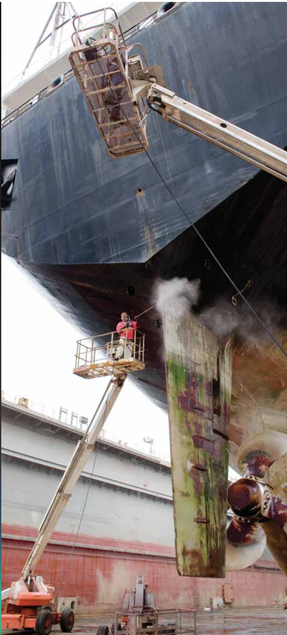
Snorkel telescopic boom lifts blast-cleaning a commercial vessel in the shipyards of Alabama, USA
